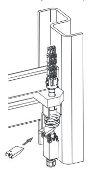
Figure 5-27. Slack/Broken Chain Sensors
