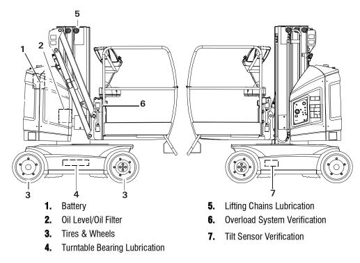
Figure 5-4. Operator Maintenance & Lubrication Diagram - 8E/20E
