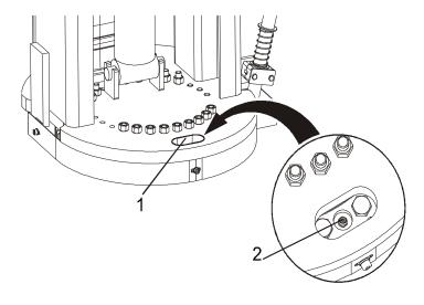
Figure 5-23. Swing Bearing Race Lubrication
