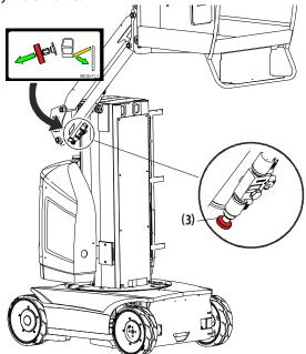
Figure 3-7. Jib Manual Descent Valve - 8E/20E
