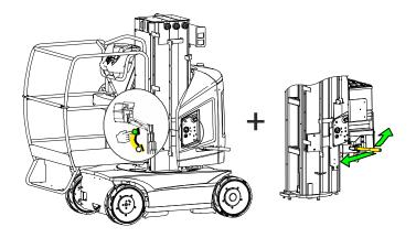
Figure 3-8. Jib Manual Lift Up Valve - 20E
