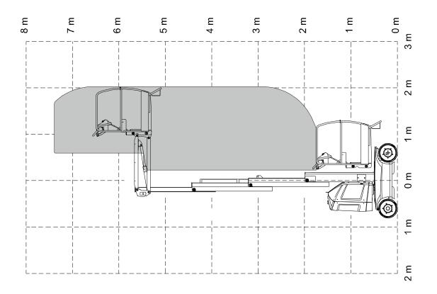
Figure 5-1. Range Diagram 8E & 8E-L/ 20E & 20E-L
