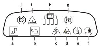
Figure 3-16. Platform Control Indicator Panel
