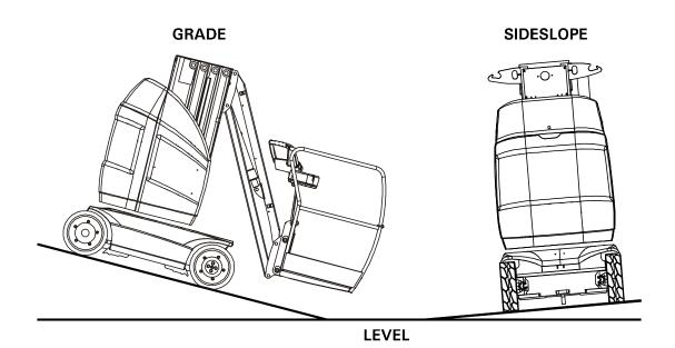
Figure 3-17. Grade and Side Slope
