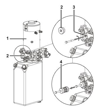
Figure 5-9. Hydraulic Filter Replacement
