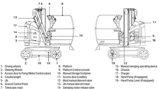
Figure 3-3. Basic Nomenclature - Machine Control Locations - 8E/20E
