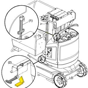
Figure 3-6. Mast Manual Descent Valve - 8E/20E
