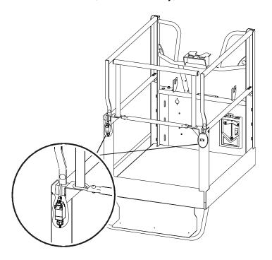
Check proper operation of the gate opening warning light and interlock. Open each gate in turn.
