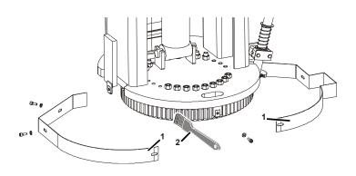
Figure 5-24. Swing Bearing Teeth Lubrication
