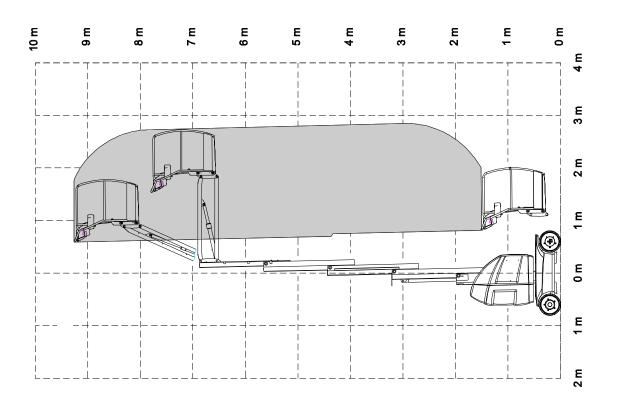
Figure 5-3. Range Diagram 10E & 10E-L - 26E & 26E-L
