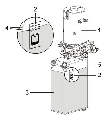
Figure 5-8. Hydraulic Oil Check - 10E/26E
