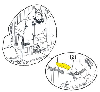
Figure 3-11. Mast Manual Descent Valve - 10E/26E
