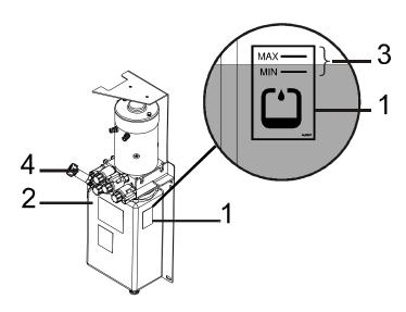
Figure 5-7. Hydraulic Oil Check - 8E/20E
