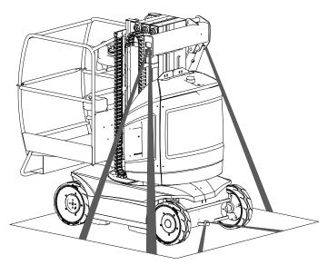
Figure 3-20. Machine Tie-Down - 8E/20E
