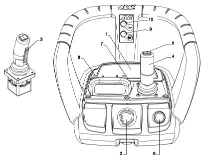
**Figure 3-15. Platform Control Station**
