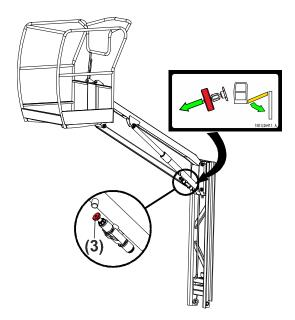
Figure 3-12. Jib Manual Descent Valve - 10E/26E
