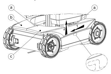
Figure 5-6. Chassis Hood Removal
