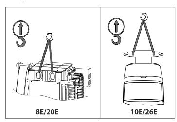
Figure 3-22. Lifting the Machine
