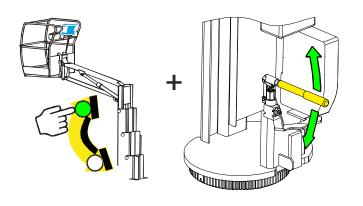
Figure 3-13. Jib Manual Lift Up Valve- 26E
